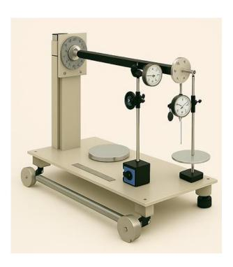
**Unsymmetrical Bending and Shear Centre Apparatus – Model KSM-075** the apparatus is designed to investigate the behavior of different sectioned beams when loading is applied outside the plane of a principal axis. The set includes cantilever beams with 'U' section, 'L' section, and rectangular section profiles.
